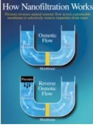
**N** anofiltration is a liquid separation membrane technology positioned between reverse osmosis (RO) and ultrafiltration. While RO can remove the smallest of solute molecules, in the range of 0.0001 micron in diameter and smaller, nanofiltration (NF) removes molecules in the 0.001 micron range.
