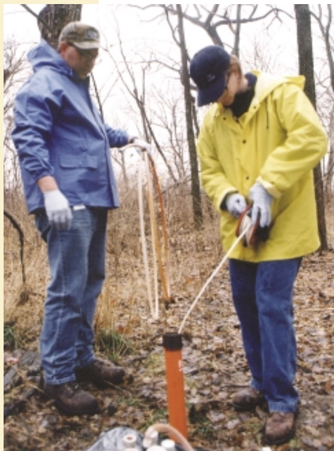
The remediation team samples groundwater using a jiggle tube so as to not disturb the American bald eagles that nest nearby.
