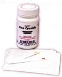
The SenSafe Cyanide test strip does not require any chemical mixing for detecting free cyanide levels in water down to 0.1 ppm. Simply collect a 50 ml sample, dip the strip into the water for 90 seconds, remove and match to the closest color to determine the concentration of free cyanide.
