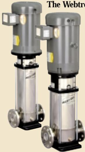
The Webtrol V Series vertical multistage pumps are designed to meet the demands of hot water applications. Features include a space-saving vertical design and a floating outer casing that allows for thermal expansion and prevents deformation due to pressure fluctuations. Capacities to 110 gpm, pressures to 360 psi and temperatures to 248° F are available.
