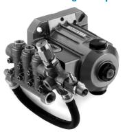
The 3SP Series direct-drive plunger pumps features V-Packing seals for long life under high pressure and a compact pressure regulating unloader for precise system pressure setting. The 3SP30G1I gas model delivers 3.0 gpm at 3,000 psi, while the 3SP35GEI electric model delivers 3.5 gpm at 2,500 psi. Both models feature a streamlined ribbed crankcase.
