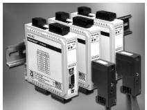
BusWorks 972PB and 973PB analog output modules deliver data from a Profibus-DP network as voltage or current signals to as many as six measurement or control devices. Typical applications involve controlling valves, drives, motors and variable level devices or providing analog signals for non-networked process instruments and control systems.
