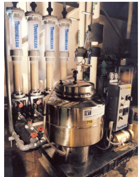
TowerKlean has several different filtration system sizes that have one to eight columns.
