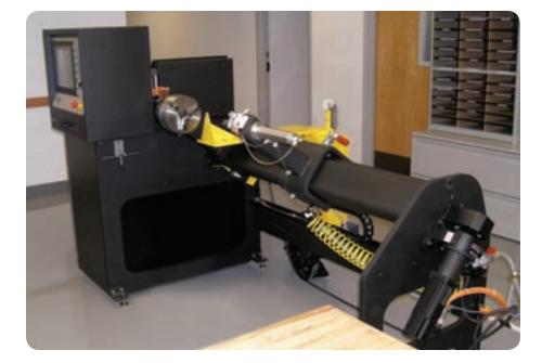
of 300 rpm. This speed creates a high enough output to ensure the filament winder does not become the bottleneck of the manufacturing process.
