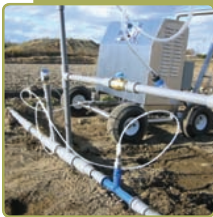
Mobile ozone generator and injection system for subsurface drip irrigation.
