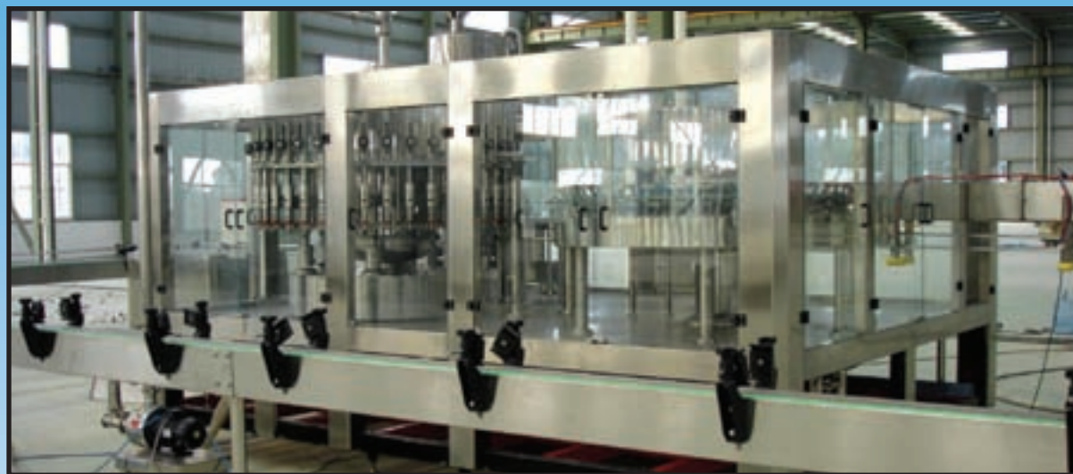
• Automated bottling systems for 250ml - 2litre, PET or glass bottles up to 20,000 BPH
