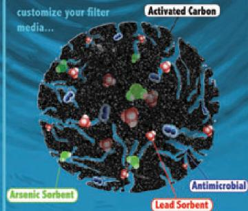
media onto carbon to create dual functionality. In this case, the acti-vated carbon reduces the organics and the bacteriostatic media inhibits the growth of bacteria.
