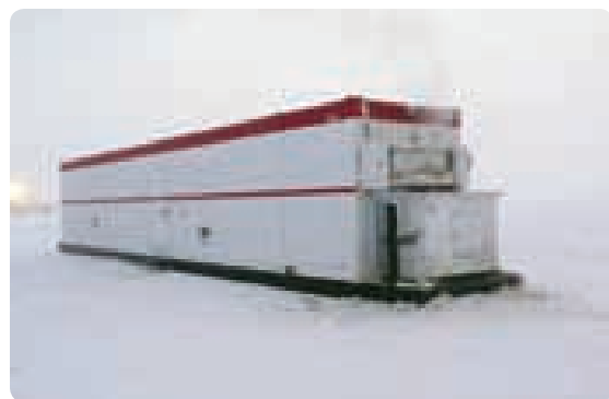
A CampWater skid-mounted nanofiltration plant operating in the Alaska Arctic.
