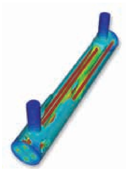
With CFdesign and the UVCalc Module, both the velocity magnitude and computed fluence rate in the UV reactor can be visualized.
