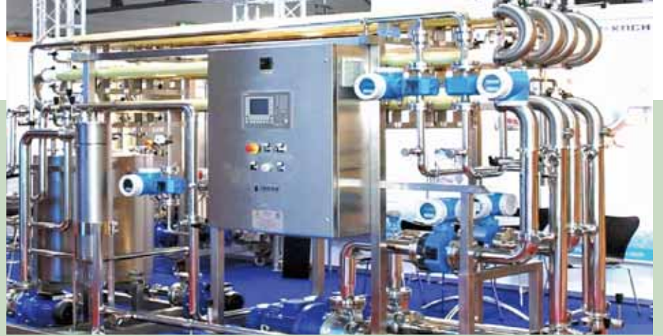
Figure 2. Membrane filtration in wine production is most commonly used to remove suspended solids and turbidity while allowing the passage of color, ethanol, flavor and aroma components.
