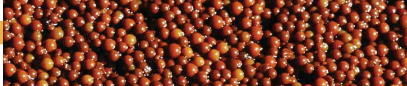
A hybrid arsenic adsorbent media consisting of particles of hydrous iron oxide that have been precipitated within an anion exchange resin bead.
