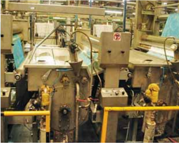
A textile manufacturing facility uses ORP to determine proper sodium hydrosulfite dosing and maintenance.
