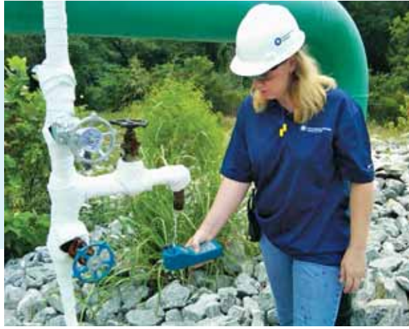
ORP is also a useful parameter when screening effluent. Here, a staff member tests effluent at a power plant.
