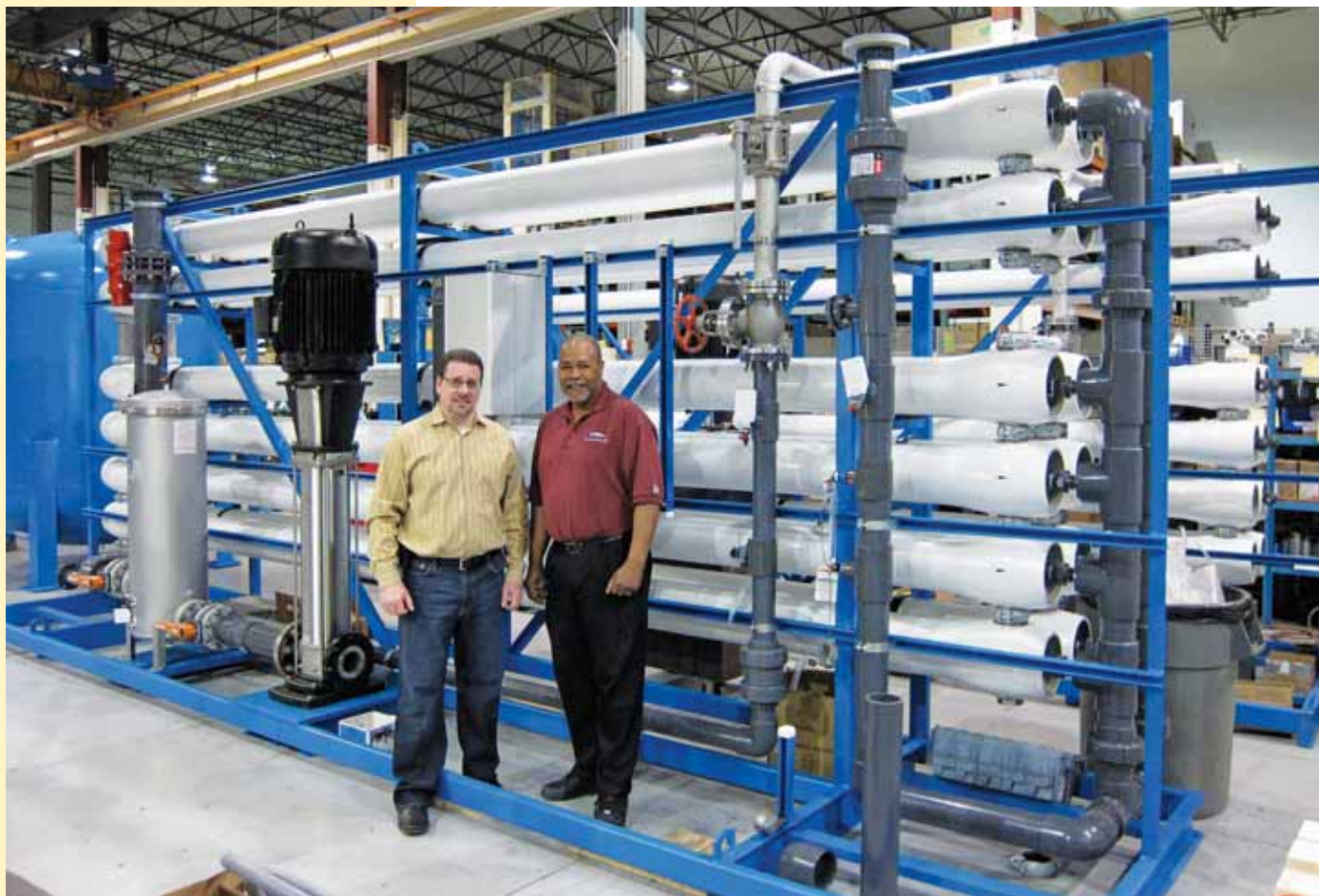
Bob Brunke, vice president of operations for Culligan Intl., and Earl Gardner, manufacturing manager for Culligan, with one of the system's 300-gpm RO units. Culligan manufactured the equipment used at the base.
