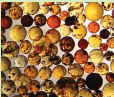
Cation resin with iron fouling
