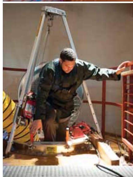
A Mondavi employee descends into a wine barrel to clean the inside walls with water that has been treated by the chlorine removal system.
