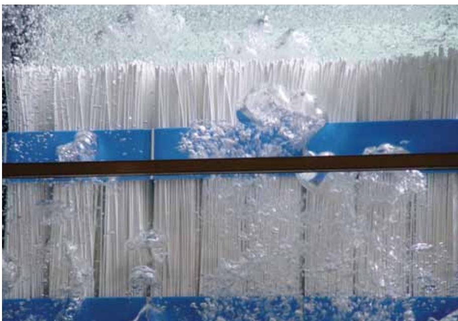
Manmade membranes are usually fashioned in the form of hollow fibers held together by a potting.
