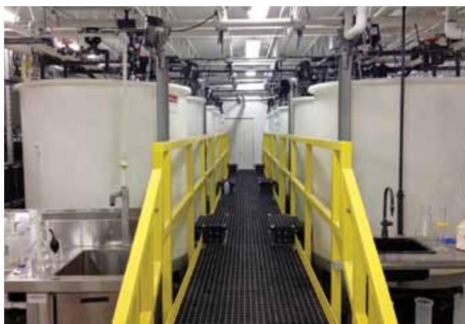
These 500-gal tanks in the Performance Lab are used to run filter testing.
