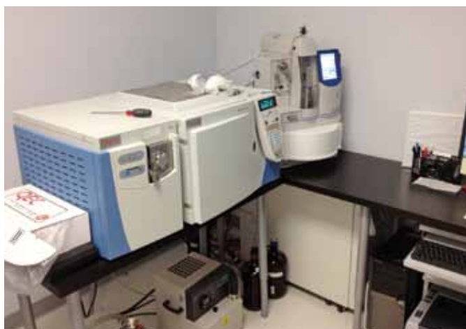
The gas chromatograph-mass spectrometer runs volatiles analyses.
