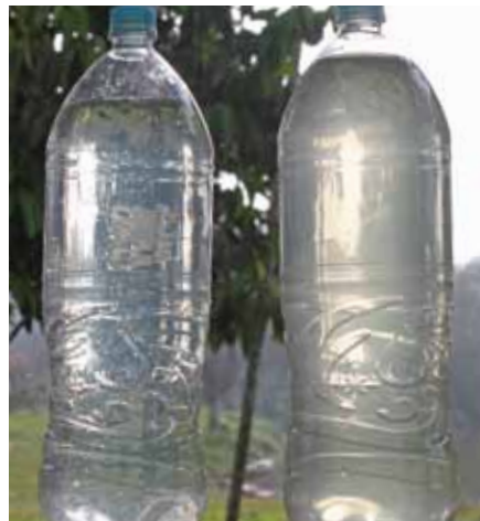
Water from a six-day-old filter (left) compared with untreated water from the Sucusari River (right) shows visibly lower turbidity levels.
