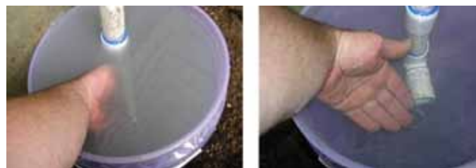
Top: Raw water at 1320 ntu (left) displays a dramatic change in quality after UF treatment. Bottom: The quality of the source water (left) visibly improves after treatment with UF (right).
