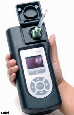
Fluorimeter with inserted syringe and sensor
