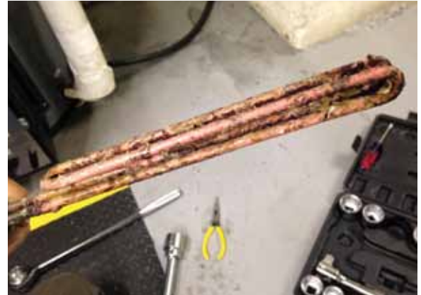
The heating elements were found to be in good working condition after 17 months of continuous operation with the catalytic system.
