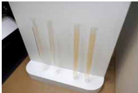
In a study, sleeves from lamp-dimming systems (left) showed less fouling than standard systems.
