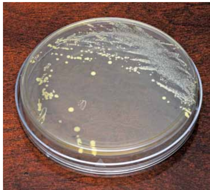
Culturing of suspected samples on bacterial culture plates, the primary method of Legionella identification, is accurate and quantitative, but can take up to 14 days.
